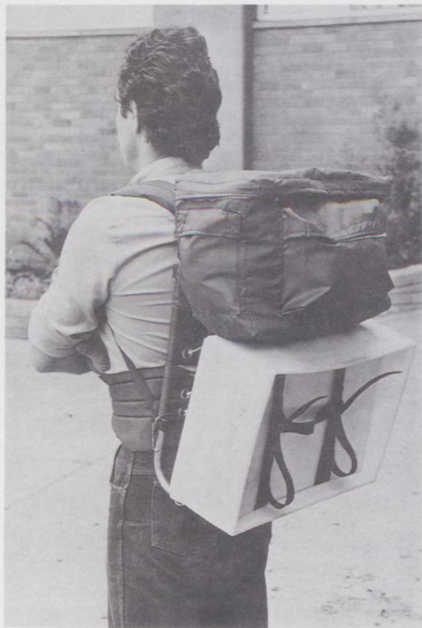
FIGURE 2.—Portable press mounted on rucksack frame with additional pockets for equipment.
