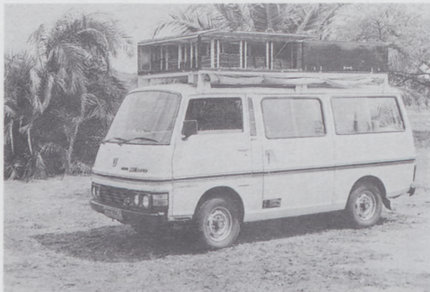
FIGURE 7.—Roofrack drier-transporter showing open front and side flaps and stowed canvas awning on awning pole box.
