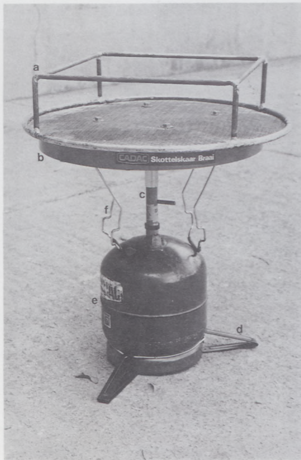
FIGURE 9. — Specimen drier showing (a) press support unit, (b) burner pan, (c) stem, (d) gas cylinder stabilizers, (e) 2,8 kg gas cylinder and (f) retaining clip handles wedged on the gas cylinder.
