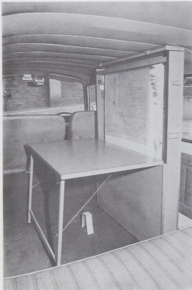
FIGURE 12.—Portable map cabinet in vehicle with front flap down to form a working surface. Note opissometer (a), attached with spring clips, for measuring distance.
